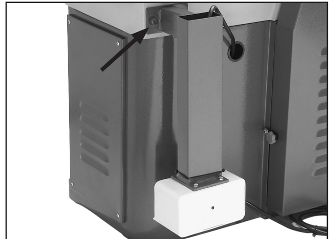
Figure 11. Location of pedestal mounting hardware (one side shown).
